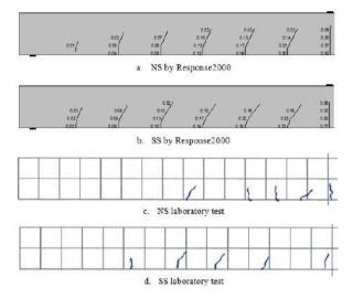
Fig. 6. Crack pattern (half of span)
